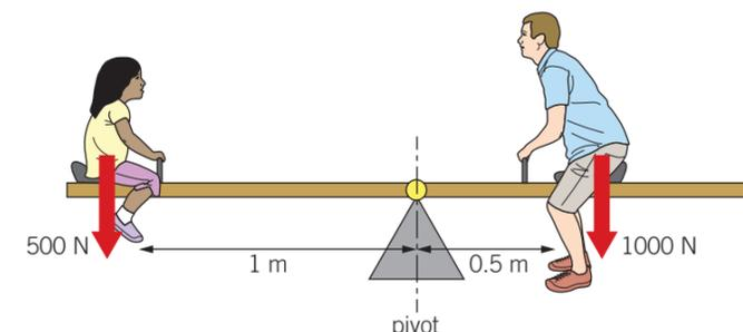
$$\begin{aligned} \text{clockwise moment} &= \text{force} \times \text{distance on the right} \\ &= 1000 \text{ N} \times 0.5 \text{ m} \\ &= 500 \text{ Nm} \\ \text{anticlockwise moment} &= \text{force} \times \text{distance on the left} \\ &= 500 \text{ N} \times 1 \text{ m} \\ &= 500 \text{ Nm} \end{aligned}$$
